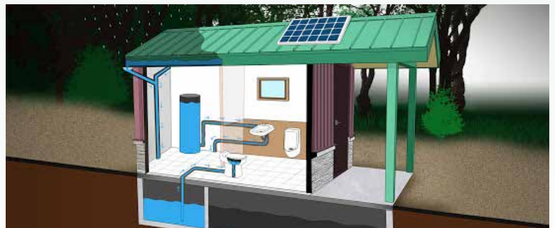
Flush Vault Latrine Comfort Station
