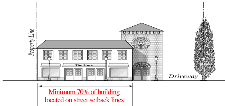
24 25 Figure 62.6.2.a.2: BUILDING PLACEMENT FOR PEDESTRIAN-ORIENTED COMMERCIAL
